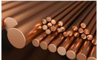
Copper alloys are metal alloys that have copper as their principal component. They have high resistance against corrosion. Thebest known traditional types are bronze, where tin is a significant addition, and brass/Gun Metal, using zinc instead.
